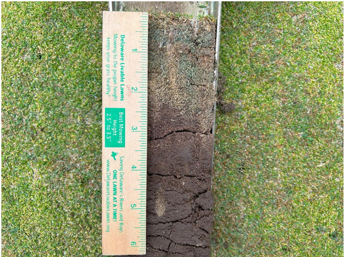
Picture 1: Notice the difference between the sandy mix in the top 2.5 – 3 inches and the native soils below. It is important to break through this interface and move sand deeper into the profile.
